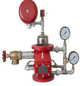
Model MN009 Alarm Check Valve is a wet pipe sprinkler system water supply check valve that makes possible the installation of sprinkler systems in buildings not subject to freezing temperatures. It is designed so that water pressure in the piping system will hold back water pressure at the valve until a significant flow of water occurs.
